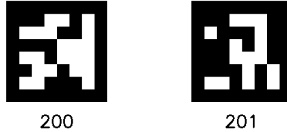
Figure 3.5: ArUco, the fiducial markers system to provide robust detection, identification, and pose estimation. Each marker has a pattern; for example, the markers with IDs 200 and 201 are represented by the patterns shown in the figure, respectively.
