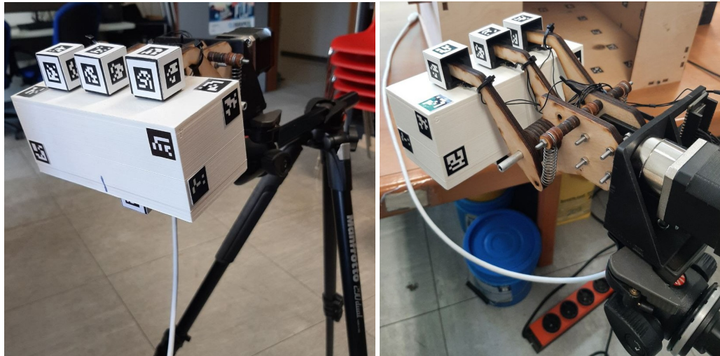
Figure 4.5: The hand-shaped gripper used for the experiments holds the test object. Each cube-like shape fingertips has different fiducial markers on each side.
