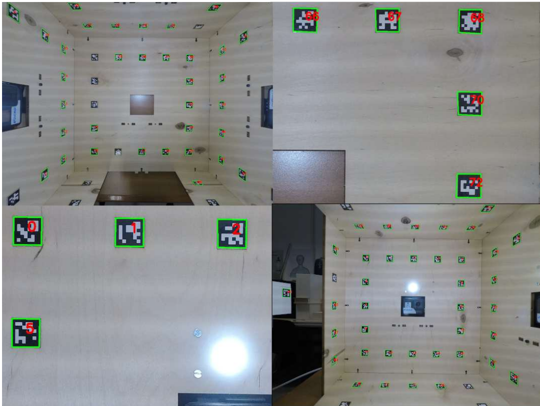
Figure 5.4: The four images shown are the outputs of the camera pose estimation process based on detected ArUco markers. In clockwise order, they correspond to the views captured by the top camera and its close-up, right camera and its close-up, respectively.
